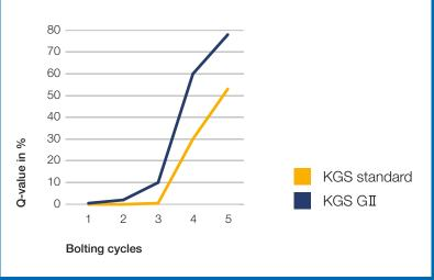
>> The quality gain after five bolting cycles can be clearly recognised in the diagram
